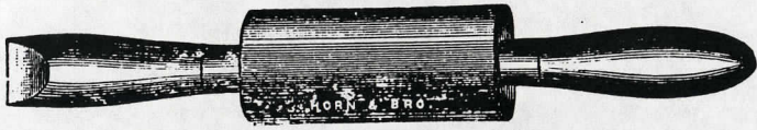
Fig. 344. —Treering Sticks. Oval and Round. Cocoa or Boxwood Centers. Solid Ironwood or Cocowood.
